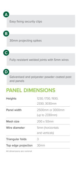
The FenceSafe Eclipse-60 was the first full Temporary Mesh Fencing system to offer all the aspects of a Rigid Mesh Fence in a temporary format. Using the Eclipse-60 by CLD Fencing Systems it provides a profiled fencing system that can be converted to permanent at the end of the project.
